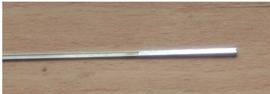
2: With a clean tip on your soldering iron (a 2mm chisel tip is ideal), tin the end of your iron tip with a little solder. Then hold the iron onto the rail, the flux will start to work its magic and the solder run into the recess. Start moving the iron tip along the rail, keeping good pressure onto the rail, allowing heat to be transferred to the rail. Once done, clean up with a file:
