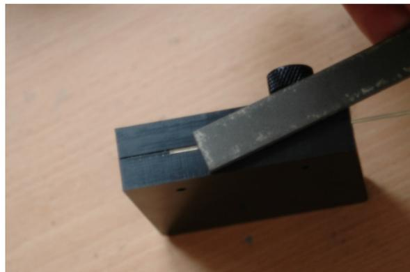
on the jig, insert the rail from the side of the jig. I recommend placing the rail half way up the jig to begin with, and file off the sharp end of the rail. Recommended use is a 'Bastard Cut' or '2nd Cut' file available from [www.britishfinescale.com](http://www.britishfinescale.com).
