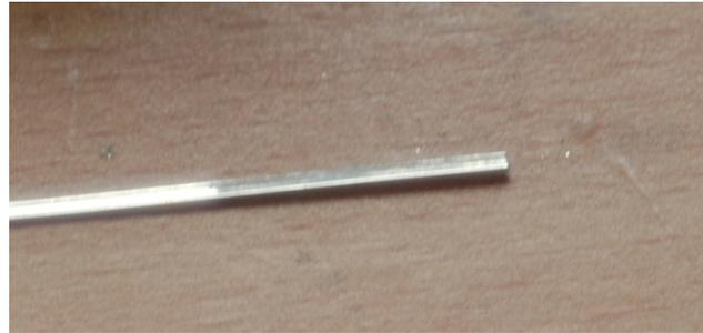
Introduce flux into the recess of the rail, about 20mm length. Wipe off any excess off the top and bottom of the rail, so that there is only flux in the recess:
