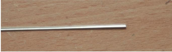
Your aim is to fill the recess of one side of the rail with solder, strengthening the rail for filing. This is a very easy job if using the correct tools. You will need a flat/chisel end soldering tip, and some flux. Fry Power Flow Flux is recommended, available from [www.britishfinescale.com](http://www.britishfinescale.com)). Without the flux, it is unlikely that the solder will flow into and along the recess of the rail:
