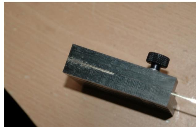
Start filing very lightly, it's easy for the file to grab the end of the rail and bend it. Once filing has started, you can increase pressure gradually:
