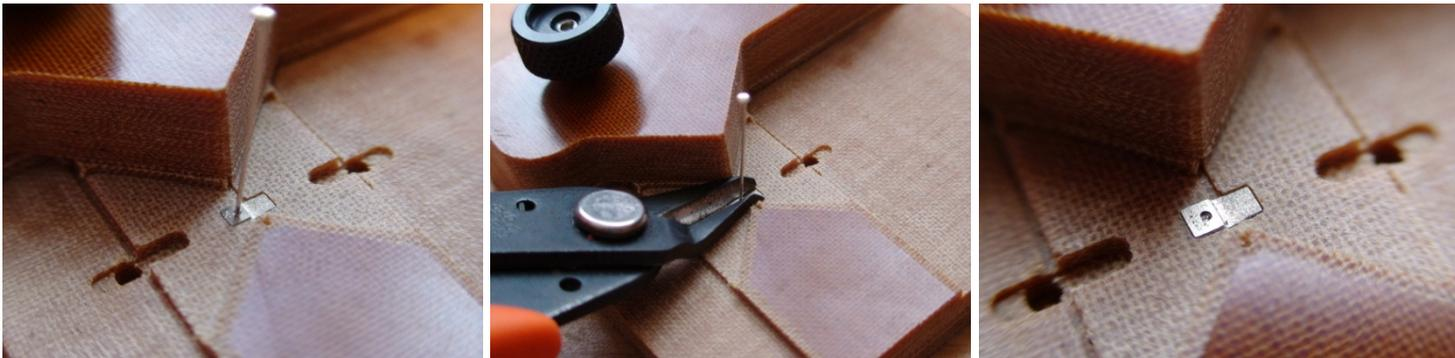
Make sure that the wire is pushed all the way to the bottom of the hole on the Jig, this will ensure that the wire/pin is the correct length. Then, using a pair of side cutters, cut the wire flush with the top of the chair plate.
