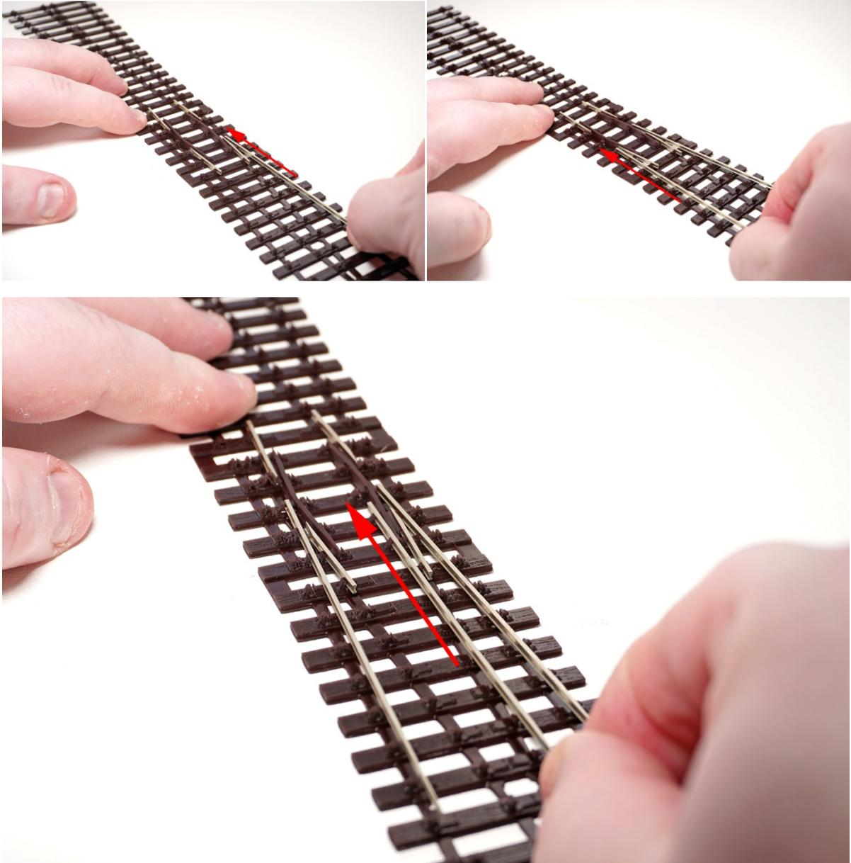
The tips of the Switch Blades should line up over the last Slide Chair as shown below:
