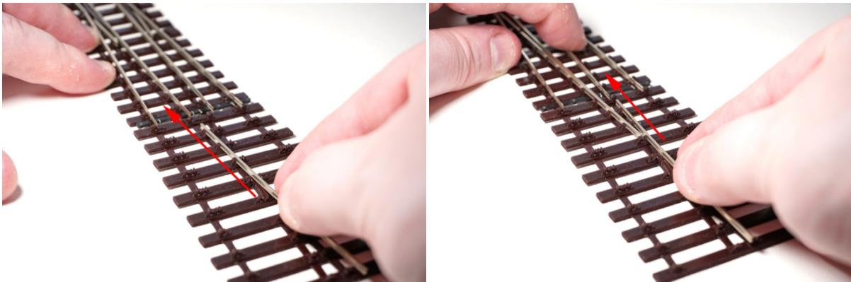
**Note:** There should be an isolating gap between the closure rails and the central 'V' rails that were previously inserted.
