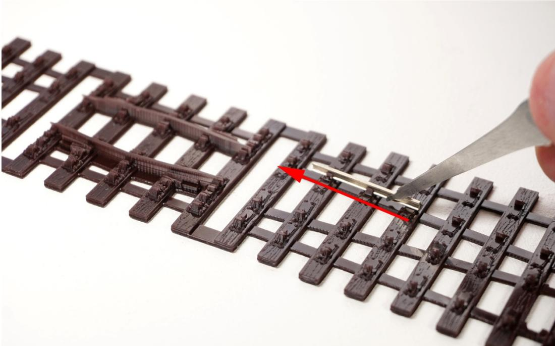
Push the V rails in until the V wedges in and cannot be pushed any further. The other end of the rail must end where shown on the downloadable template.
