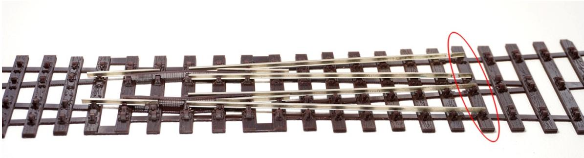
Repeat for the other side. The 4 **outermost** Switch Blades should make contact with its opposing Switch Blade right at the knuckle of the 'Diamond' (the very centre of the formation).
