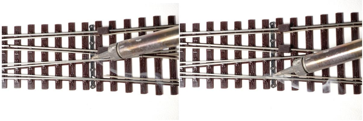
With the 4 Switch Blades now soldered, the same can be repeated for the 4 Switch Blades on the opposite side of the Slip.
