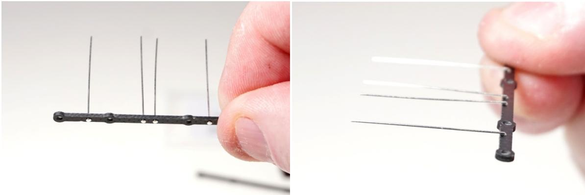
Make sure that the 4 headed pins are pushed all the way through until the heads of the pins are flush with the bottom of the tie bar. Then bend both pins by 90 degrees so that they face forward as shown above.
