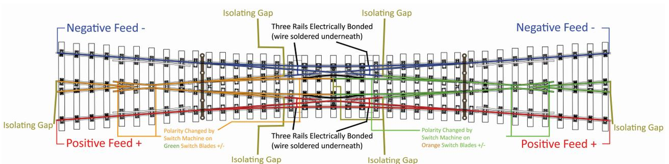
Each of the 4 'V' Rails in the middle of the Slip should be electrically bonded to its adjacent Switch Blade and Stock Rail by soldering a small piece of wire between them under the rails at the point shown in the diagram.
