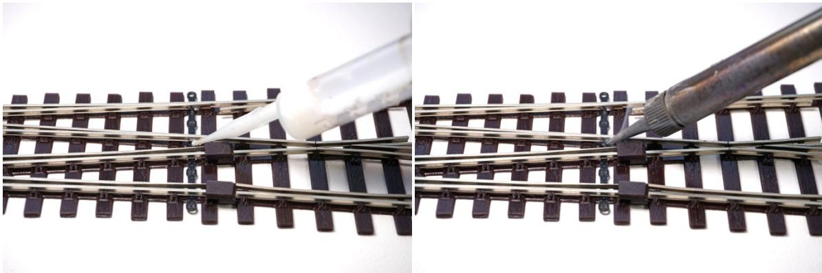
The same can then be repeated for the other two Switch Blades. Move the 'Spacers' to the other Stock Rails, which will hold the two Switch Blades that you just soldered, open at the correct gap.
