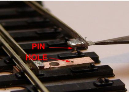
The tie bar should be placed into position between the timbers on the base where there is a slit for the switch machine wire.
