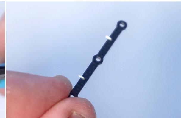
The pins can then be cut short leaving about 2 – 3mm of length as shown above.
