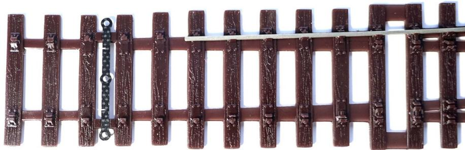
Once the Tie Bar is in place, both Stock Rails can then be inserted from either end of the turnout. Care must be taken so each Stock Rail slides over the Tie Bar. The Tie Bar must be free to slide under the Stock Rails when operating the Switch Blades.
