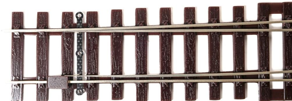
Soldering is done while the Switch Blade sits flush against the Stock Rail as this ensures best alignment. If you notice a gap between Switch Blade and Stock Rail, this can be taken up by squeezing them together at the top of the rail head with a small pair of tweezers, whilst soldering.
