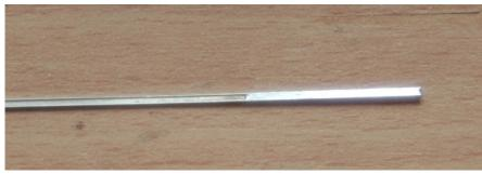
2: With a clean tip on your soldering iron (a 2mm chisel tip is ideal), tin the end of your iron tip with a little solder. Then hold the iron onto the rail, the flux will start to work its magic and the solder run into the recess. Start moving the iron tip along the rail, keeping good pressure onto the rail, allowing heat to be transferred to the rail. Once done, clean up with a file:
