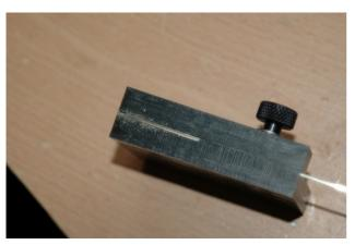
Start filing very lightly, it's easy for the file to grab the end of the rail and bend it. Once filing has started, you can increase pressure gradually:
