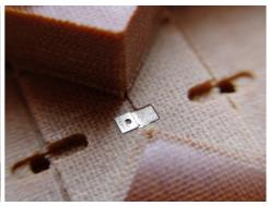
Make sure that the wire is pushed all the way to the bottom of the hole on the Jig, this will ensure that the wire/pin is the correct length. Then, using a pair of side cutters, cut the wire flush with the top of the chair plate.
