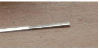
Introduce flux into the recess of the rail, about 20mm length. Wipe off any excess off the top and bottom of the rail, so that there is only flux in the recess:
