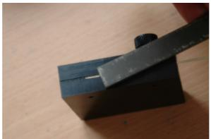
on the jig, insert the rail from the side of the jig. I recommend placing the rail half way up the jig to begin with, and file off the sharp end of the rail. Recommended use is a 'Bastard Cut' or '2nd Cut' file available from www.britishfinescale.com.
